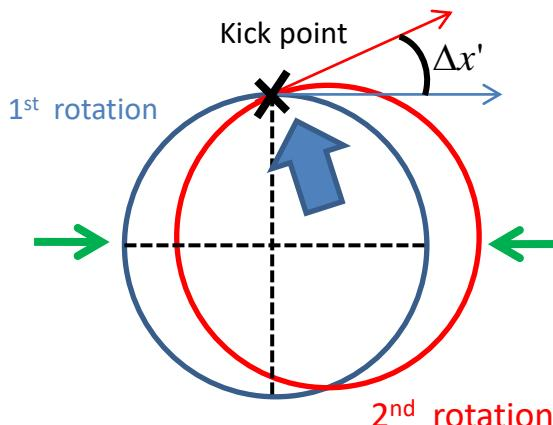
Difference between the 1<sup>st</sup> and 2<sup>nd</sup> rot. orbits is maximized at 1/4 and 3/4 rot. points by this kick. And its value is  $\rho \Delta x'$ .
